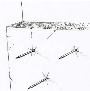
Insulation can be impaled immediately but maximum strength of adherence is achieved after 24 hours.
