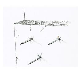
Impale the insulation material on the pins
