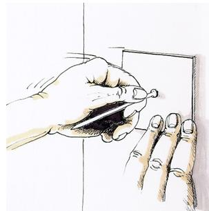
Place the hanger in the required position and press the base against the surface to be insulated
