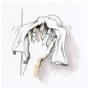
Apply at temperature range +15°C to +25°C (+60°F to +77°F). Surfaces should be clean and dry, free of dust, grease, oil and any other loose matter. Do not use degreasing products. Not for use in application likely to make contact with chlorinated, cетonic or esther solvents.
